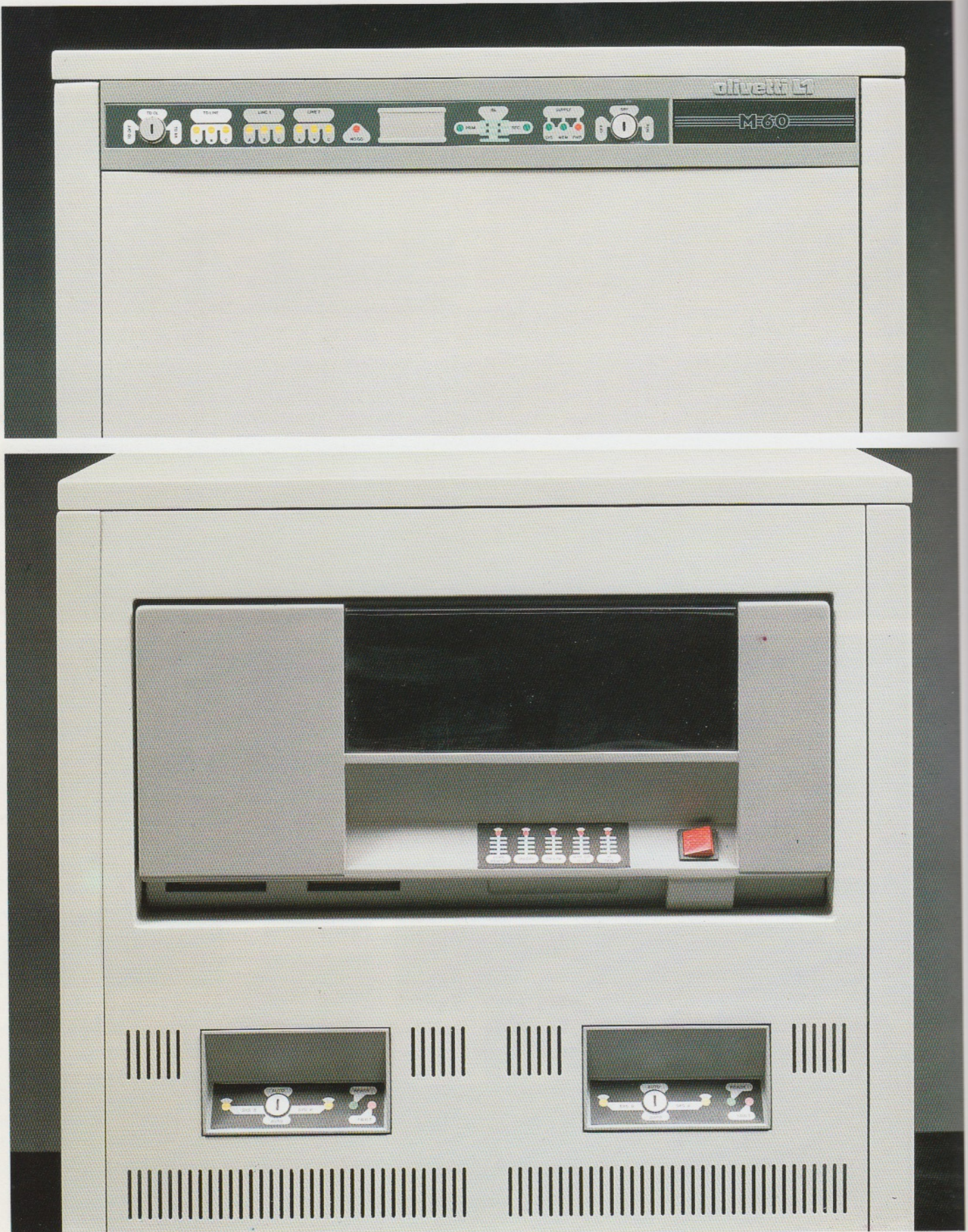
The M60 concentrator and the SB2 ribbon unit.
